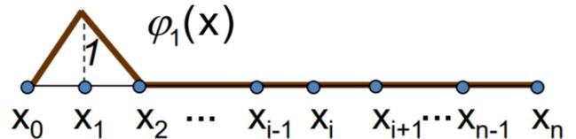
$$\varphi_i(x) = \begin{cases} \frac{x - x_{i-1}}{x_i - x_{i-1}} & \text{si } x \in [x_i, x_{i-1}] \\ \frac{x - x_{i+1}}{x_i - x_{i+1}} & \text{si } x \in [x_i, x_{i+1}] \\ 0 & \text{si } x \in [x_0, x_{i-1}] \cup [x_{i+1}, x_n] \end{cases}$$
