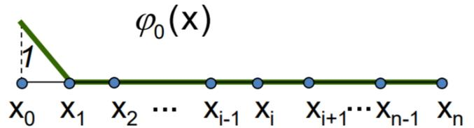
$$\varphi_1(x) = \begin{cases} \frac{x - x_0}{x_1 - x_0} & \text{si } x \in [x_0, x_1] \\ \frac{x - x_2}{x_1 - x_2} & \text{si } x \in [x_1, x_2] \\ 0 & \text{si } x \in [x_2, x_n] \end{cases}$$
