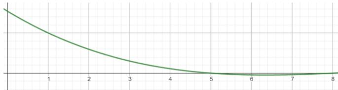
$$L_2(x) = \frac{(x - x_1)(x - x_3)(x - x_4)}{(x_2 - x_1)(x_2 - x_3)(x_2 - x_4)} = \frac{(x - 1)(x - 8)(x - 14)}{(4)(-3)(-9)} = \frac{(x - 1)(x - 8)(x - 14)}{108}$$
